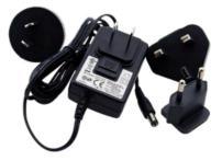
• Table-Top Power Supplies are similar to wall transformers but they get their name because they sit on a table rather than in a wall receptacle. The advantage of a table-top supply is that you can cut the AC power cord's plug and wire it in with the rest of your AC power. The barrel connector must be cut off in order to attach to the ESS's screw terminals. The supply shown in the picture uses a standard computer style of power cord with a "C13" plug.
